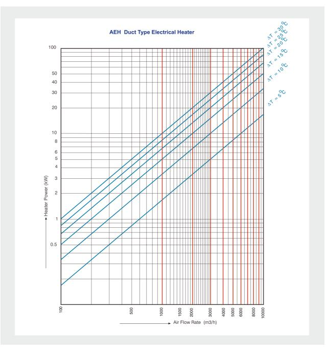
NOTE: Heater face velocity must be greater than 2m/s.
